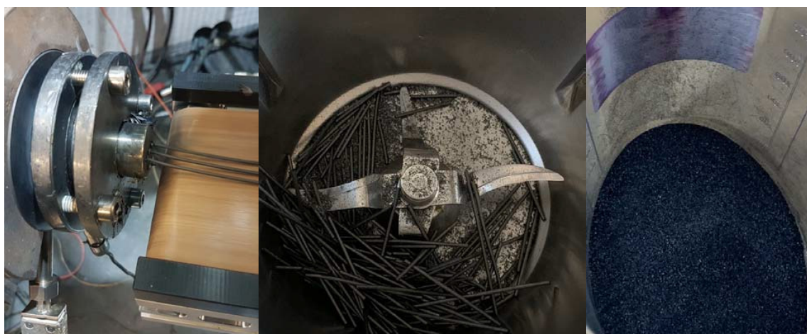
Figure 2: Production Process of Highly Filled Carbon Compounds for Additive Material Extrusion
